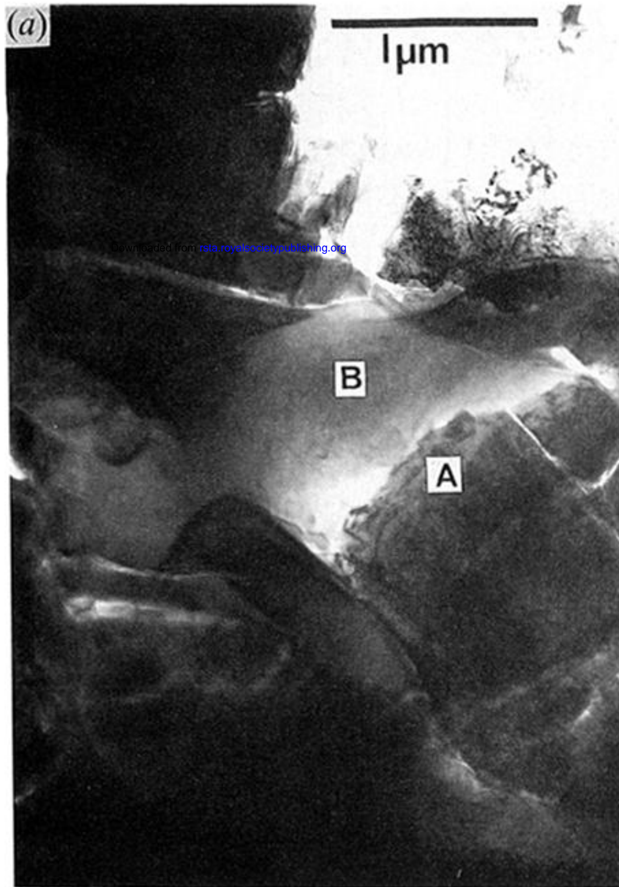
Figure 3. (a) Detail of multiple cementation in a web. An early pure calcite cement, A, has been fractured and a new Fe–Mn calcite cement, B, precipitated. Note the more complex defect structure in the older, deformed cement. TEM micrograph of Web from Alvin 2948-5V1. (b) Multiple fracture and cement events within a web structure. An early event has fractured Grain A and then sealed it with K-feldspar growth. K. A later event associated with calcite cementation has fractured both the original grain and the first cement. BSE image of specimen from Leg 66 493-100–105 cm.
